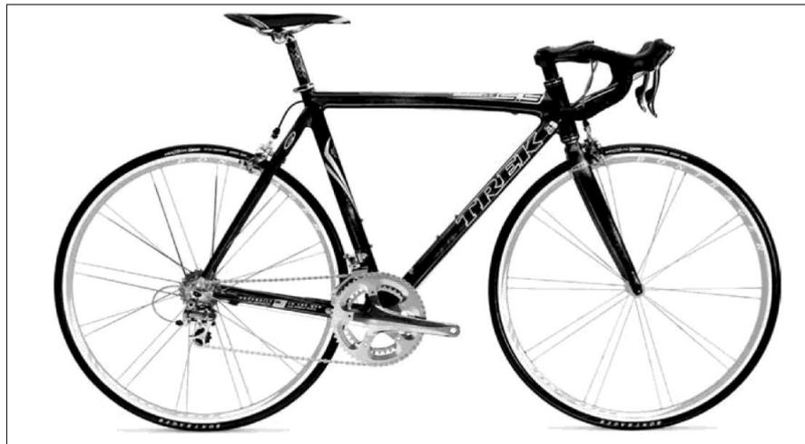
Figure 22 Carbon fiber-reinforced epoxy bicycle frame [26].
