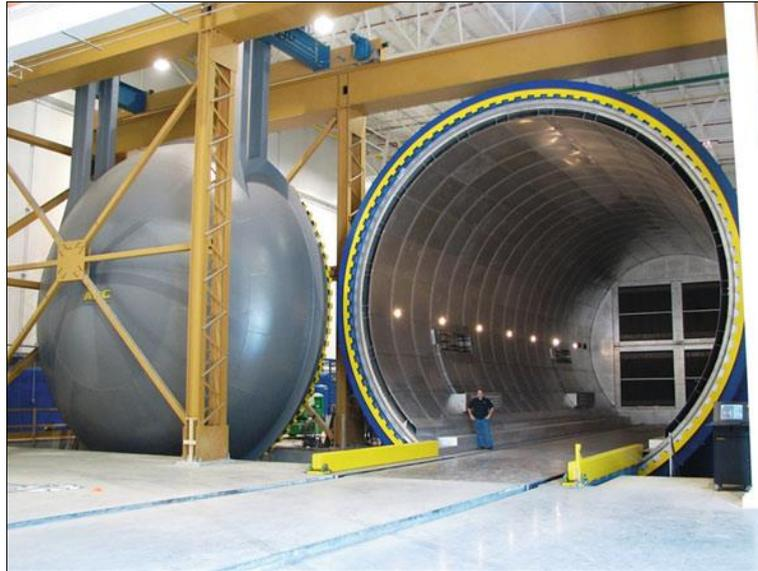
Figure 16 A large autoclave that is used to make the wings of Boeing 787 [21]
