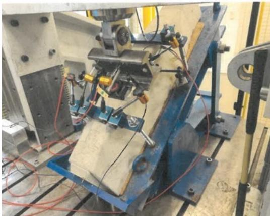
Test setup for repeated load test according to DIN EN 13146-4
